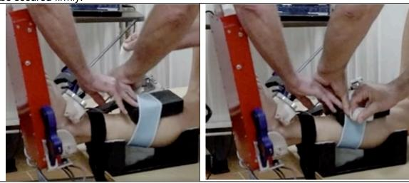
8. The examiner should place their knee against the bottom of the dorsal foot pad while pulling up on the load handle with 50-100 N force. The examiner should tighten the dorsal foot pad, then the heel pads and repeat until the device is secure.
